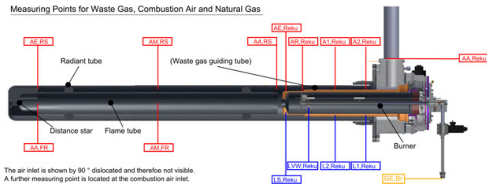
Fig. 11. Overview of all measuring points (red for waste gas, yellow for natural gas, blue for combustion air).
